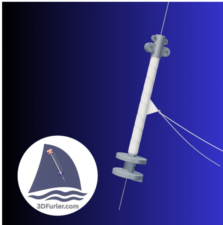
Figure 18 Sail furled on the 3D Furler – wrap extra turns before attaching furler line.
